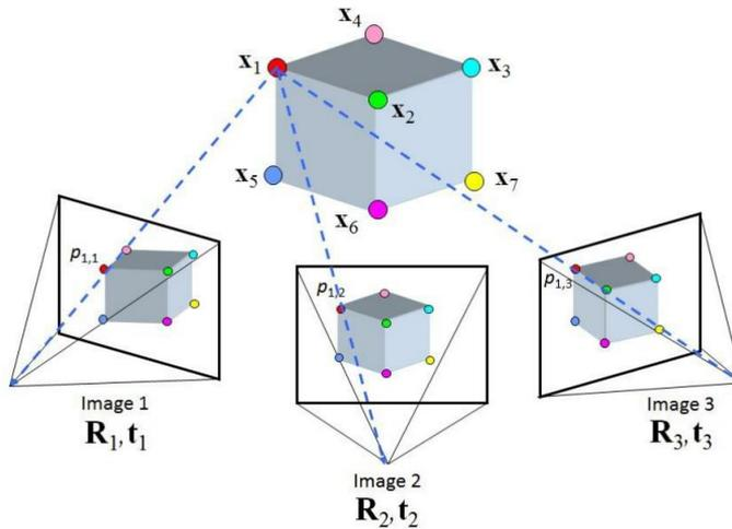
Figure 2 – Structure from Motion [5]
