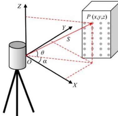
Figure 8 – Measuring principle of the terrestrial laser scanning [14]
