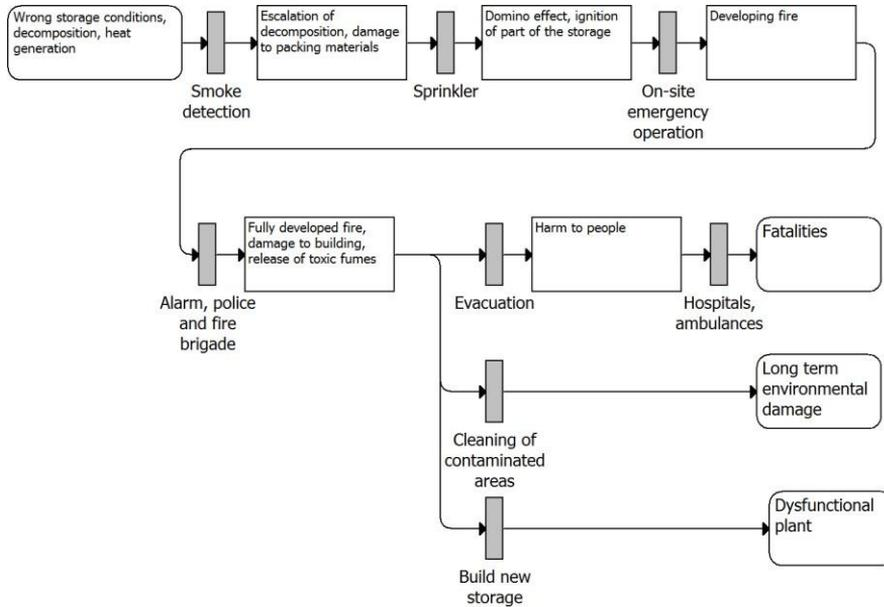
Figure 9 - Example for an Safety Barrier diagram for a warehouse fire scenario
