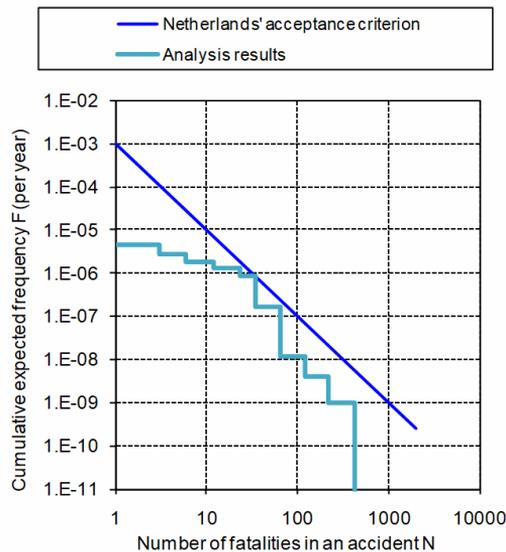
Figure 6 - example for FN-curve
