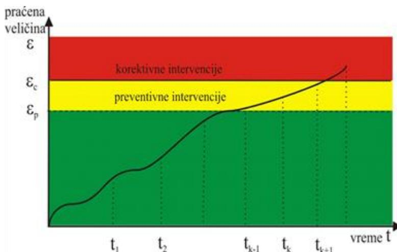
Figure 1 – The behavior of the system in time:  $\varepsilon_p$  border on which are performed prevention interventions,  $\varepsilon_c$  limit where the running corrective intervention,  $t$  – time moments in which to perform diagnostics
