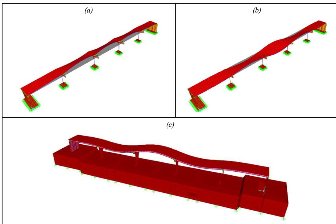
*Fig.14. Numerically predicted modes: (a) Transverse mode of S1-NB3-M2 model; (b) Torsional mode of S1-NB3-M2 model; (c) Bending mode of S5-NB3-M2 model*
