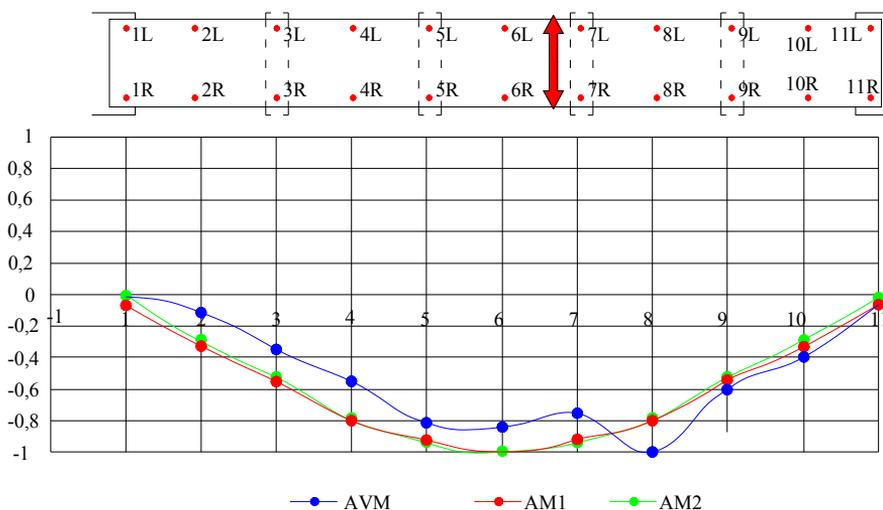
Fig.16. Experimentally and mathematically identified first transverse mode shapes
