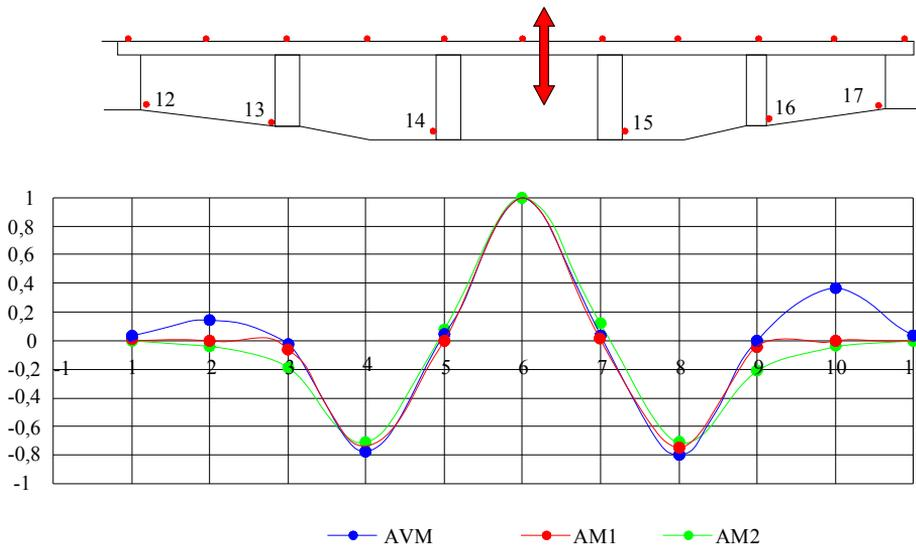
*Fig.15. Experimentally and mathematically identified first vertical mode shapes*
