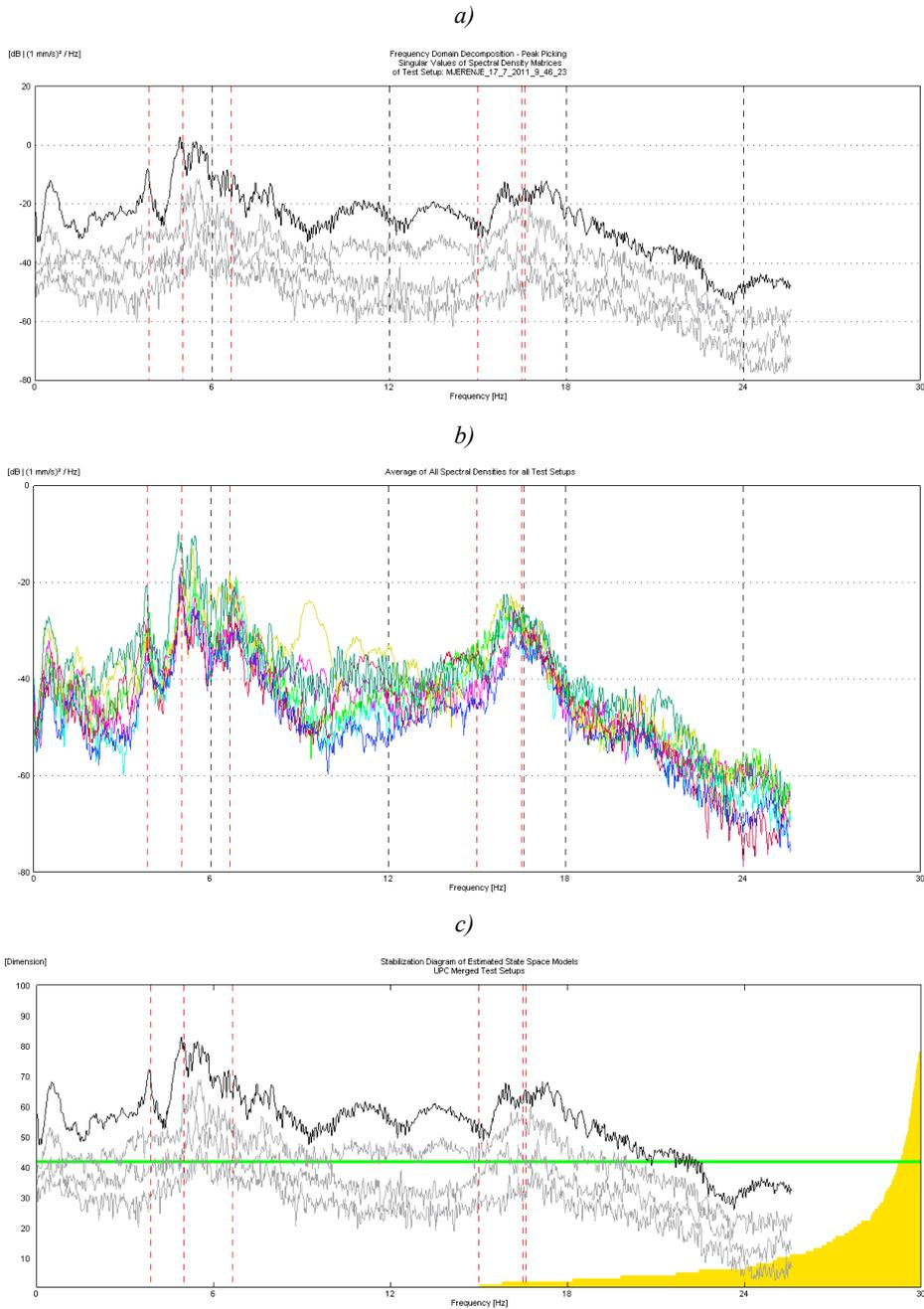
*Fig.11. Dynamic characteristics attained from the test using EFDD and SSI methods: (a) singular values of spectral density matrices, (b) average of auto spectral densities, and (c) stabilization diagram of estimated state space model.*
