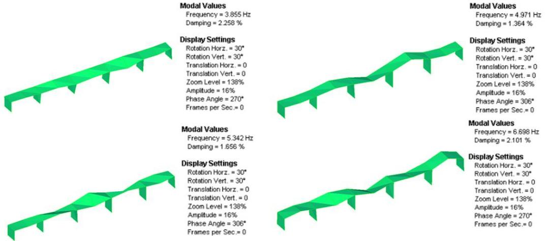
Fig.12. Experimental modal parameters attained from the test setup
