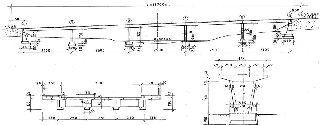
Fig.2. Elevation and cross-sections of the bridge
