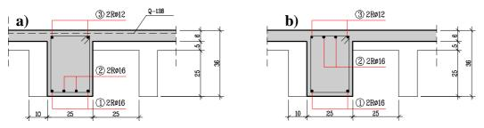
Figure 24. The new beam reinforcement plan: transversal cross-sections: a) in the span; b) in the support zone
