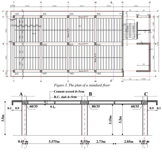
Figure 4. Cross-section of a standard floor
