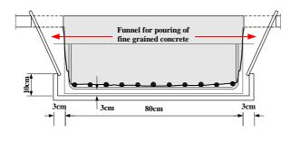
Figure 19. Placing of new cover on the down part of the beam
