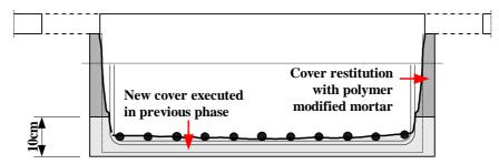
Figure 21. Applying the new protective cover on the side surfaces of the beam
