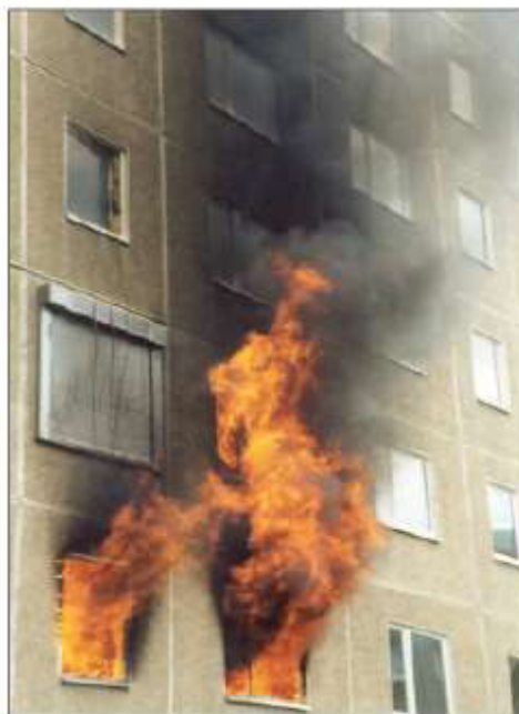
After 20 minutes „flash-over“ 2nd floor
