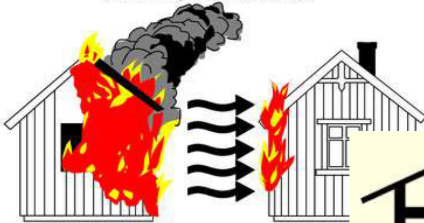
Spread of Fire by Radiation (From a Burning Timber House to Another)
