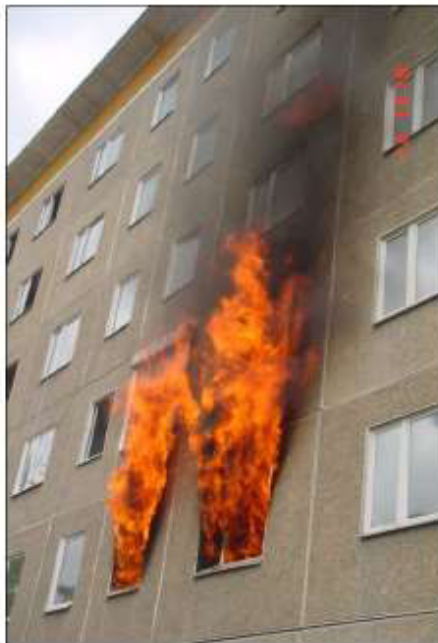
After 12 minutes „flash-over“ 1st floor
