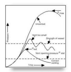
Used for the design of deflagration protection (venting, suppression, Containment)
