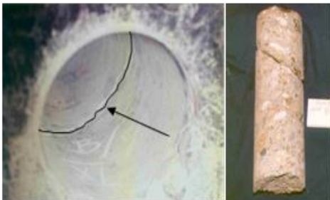
Figure 7. Inner delamination of concrete in the column
