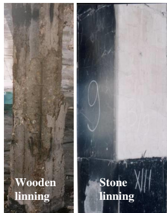
Figure 18. Influence of type of decorative layer type on the fire damage degree of concrete columns
