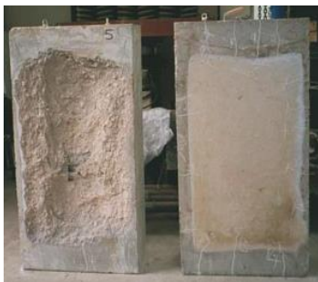
Figure 11. A view of OC (left - explosive spalling) and PPFRFRC (right) after exposing to elevated temperatures
