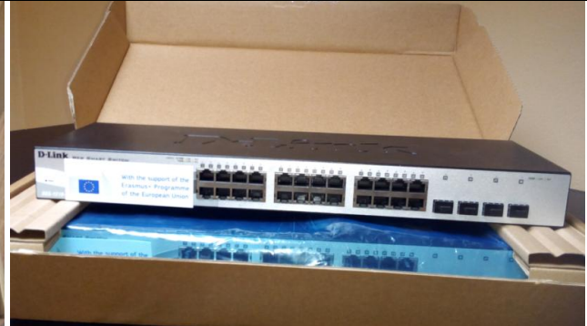
17. D-link DGS-1210-28 network switch (2 pieces)
