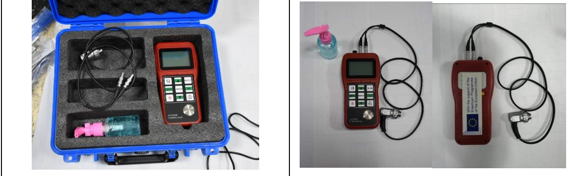
16. The compact ultrasonic thickness meter for homogeneous materials (1 pcs)
