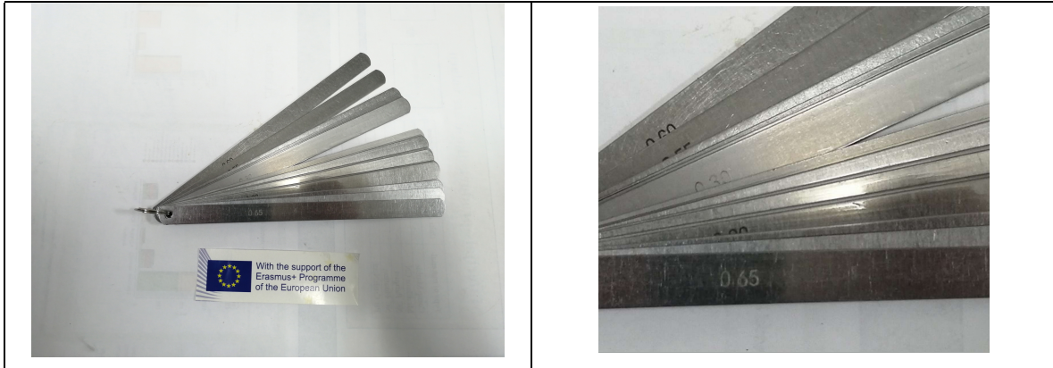
21. Precision feeler gauges (thickness 0.03-1.00, length 100 mm) (1 pcs)
