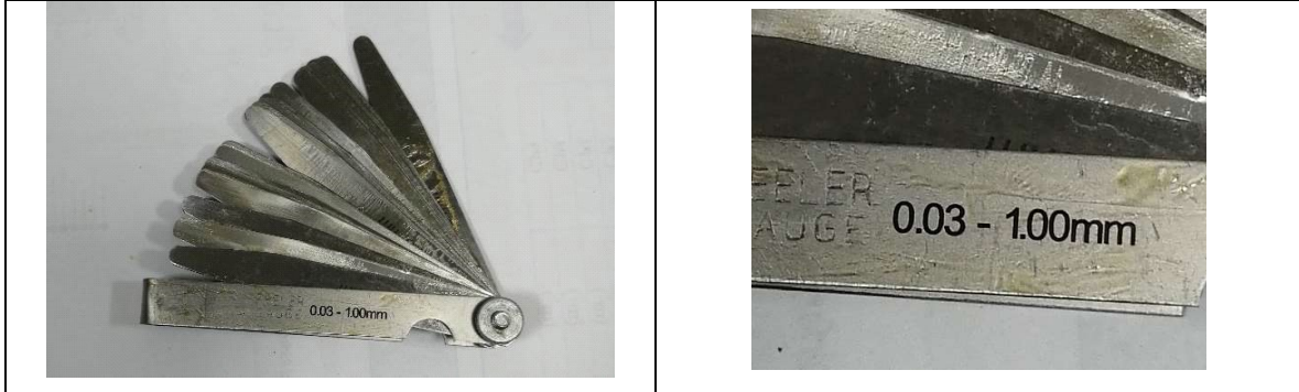
19. Precision feeler gauges (thickness 0.05-1.00, length 200 mm) (1 pcs)
