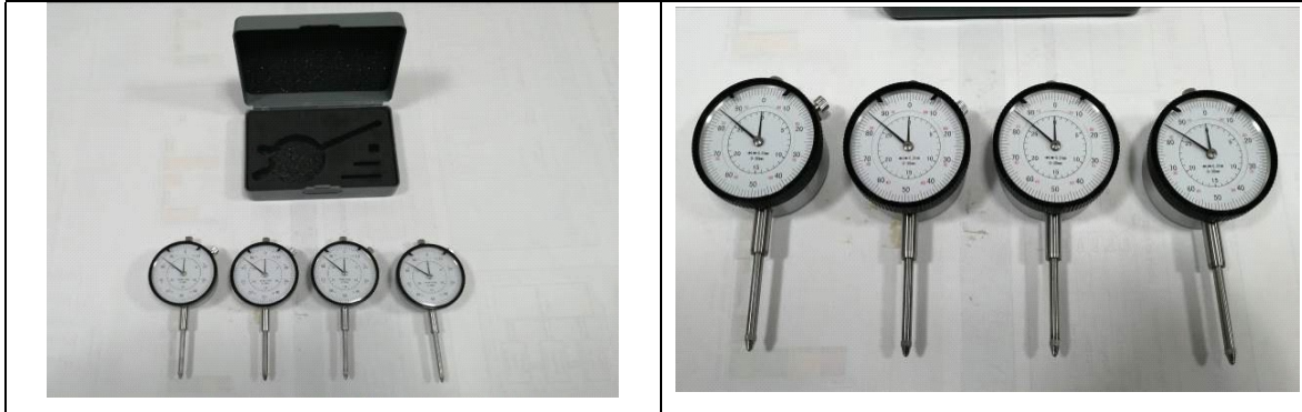
26. Comparator (precision 0.01 mm, rang 0-3 mm, analog) (4 pcs)
