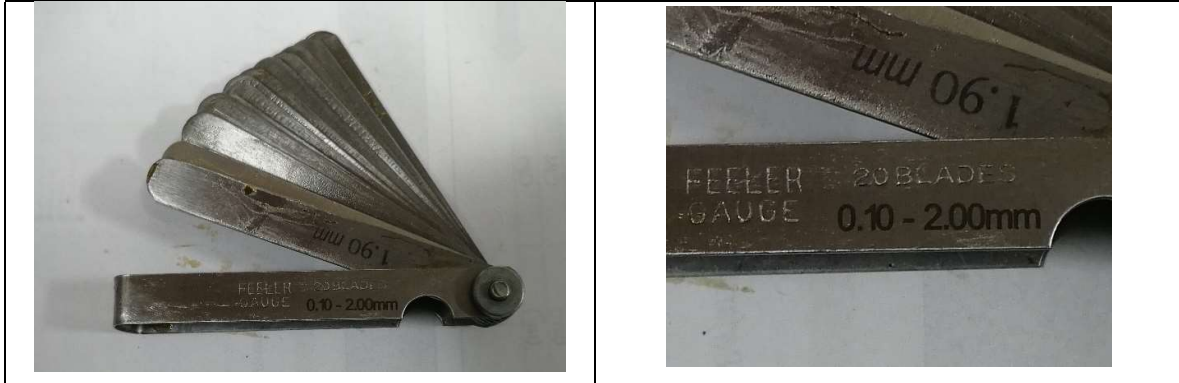
20. Precision feeler gauges (thickness 0.10-2.00, length 100 mm) (1 pcs)
