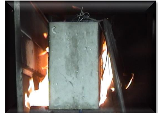
Fire testing of beam specimen
