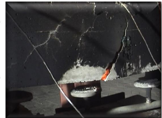
Fire penetrating cracks in beam specimen
