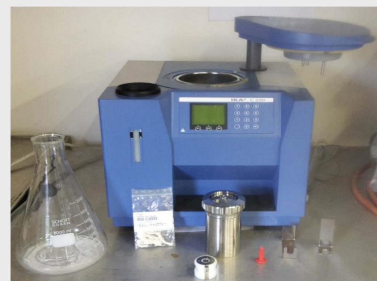
Bomb calorimeter parts
