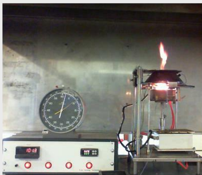
Cone calorimeter setup (time to ignition)
