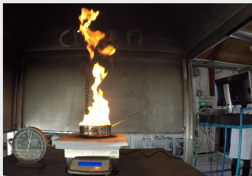
Liquid pool fire setup
