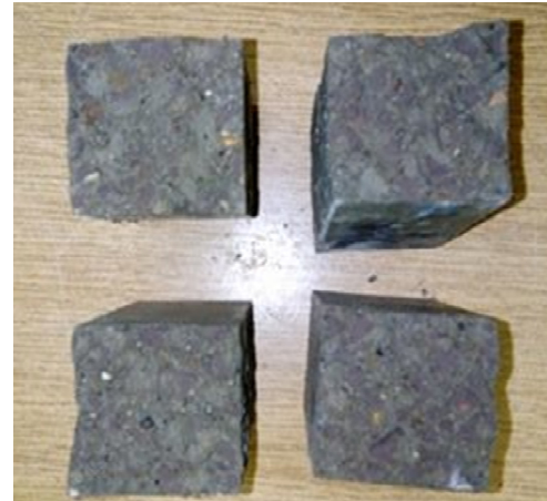
Fig. 4. Crushed aggregate concrete prisms
