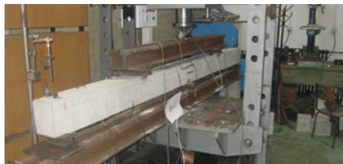
Fig. 1. Experimental setup of the tested beams
