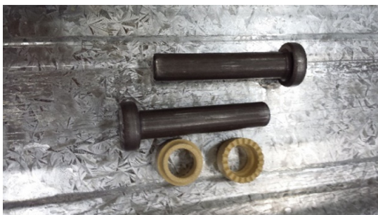
Fig. 1. Headed shear connectors with ceramic ferrule
