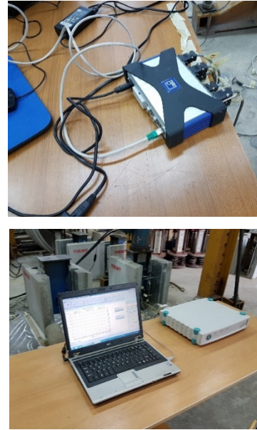
Fig. 7. Testing equipment (HBM Quantum and HBM Spider 8)
