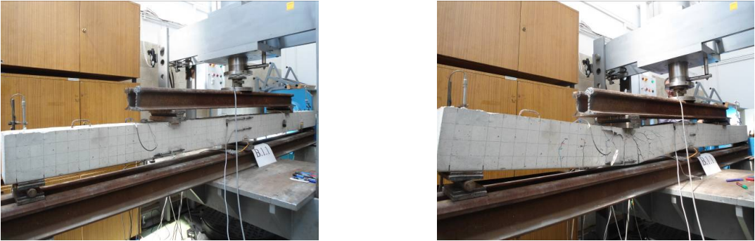
Fig. 4. Disposition of continuous beam in the testing phase
