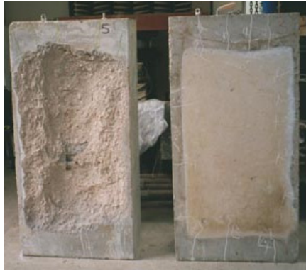
Fig. 13. A view of OC (left - explosive spalling) and PPFRC (right) after exposing to elevated temperatures
