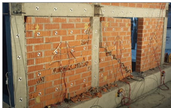
Fig. 10 Damage to the infill of the MODEL 1
