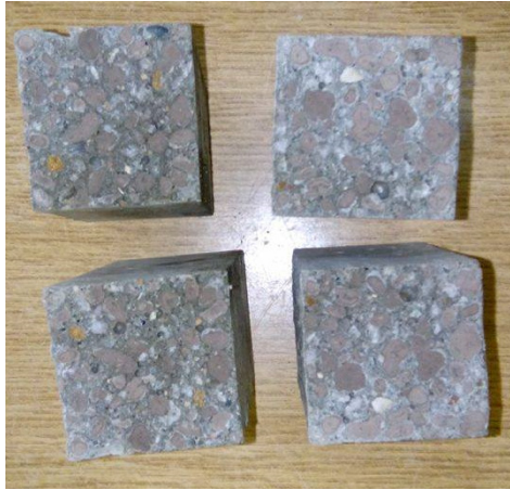
Fig. 3. Pelletized aggregate concrete prisms
