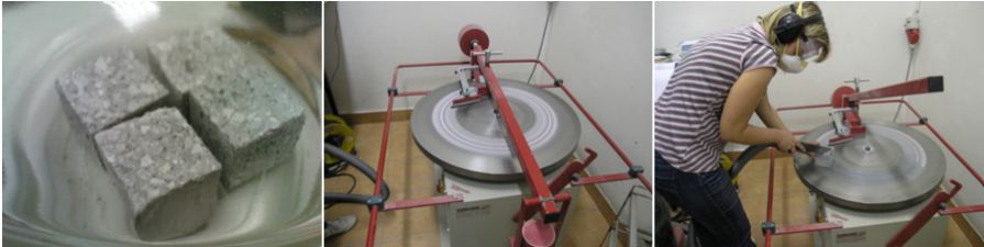
Fig. 6 Abrasion resistance equipment – Böhme test
