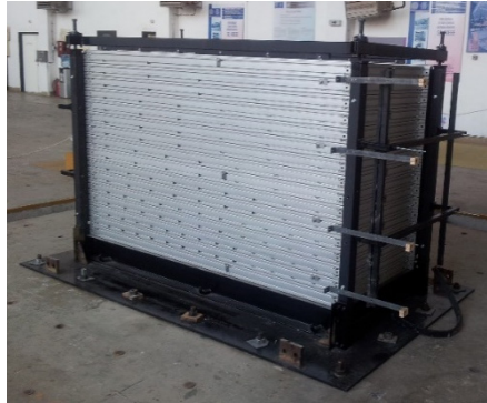
Fig. 6. The constructed laminar box
