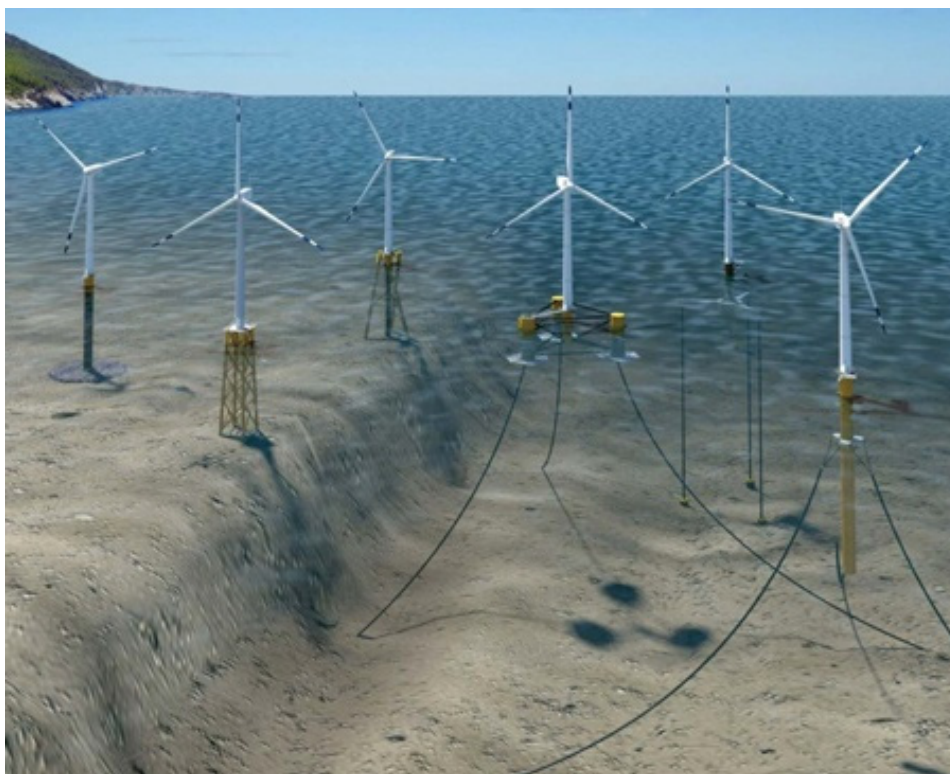
Fig. 2. Offshore wind turbine support structures. Monopile, jacket, twisted jacket, semisubmersible, tension-leg platform, and spar buoy. Courtesy of Smith et al. (2015).
