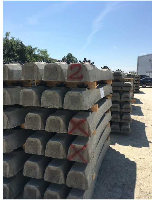
Fig. 2. Taking over of sleepers and fastening in the factory Rajshwellen Serbia
