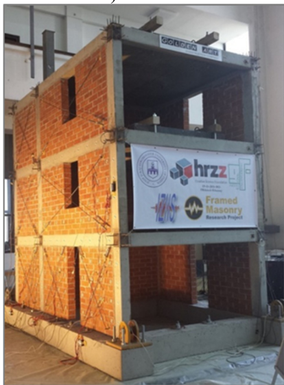
c) Instrumentation set up – view on the shaking table Fig.7 Instrumentation set up of the models
