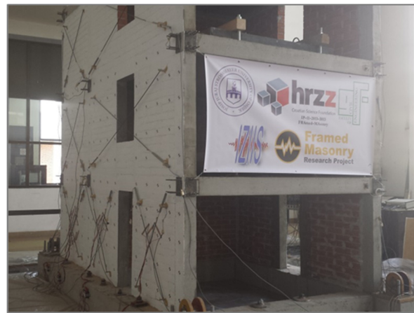
c) Instrumentation set up – view on the shaking table Fig.7 Instrumentation set up of the models
